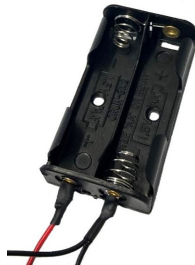
Fig. 16: Ready connected battery holder
