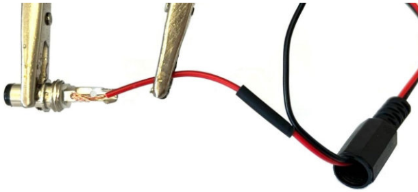
Fig. 14: Soldering the hollow connector to the cable
