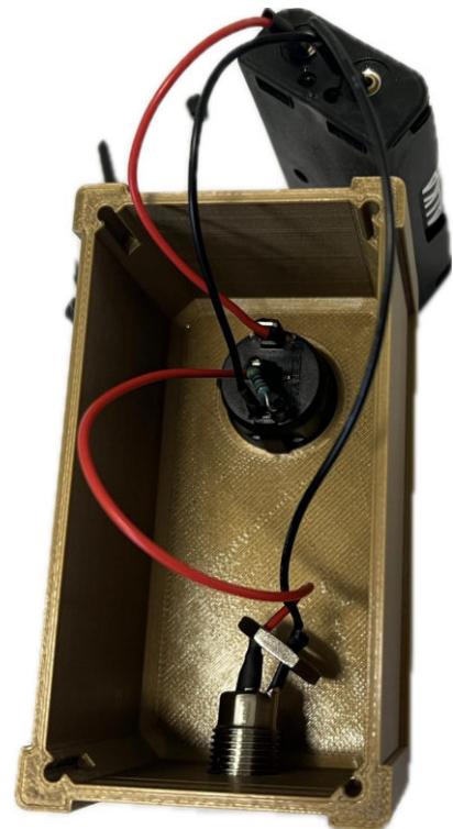
Fig. 21: DC-Socket in the cover
