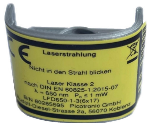
Fig. 8: Laser warning sign glued to the laser plate
