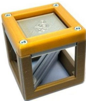
Fig. 11: Screwed together beam splitter
