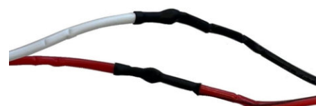
Fig. 13: Shrink tubing over the solder joints
