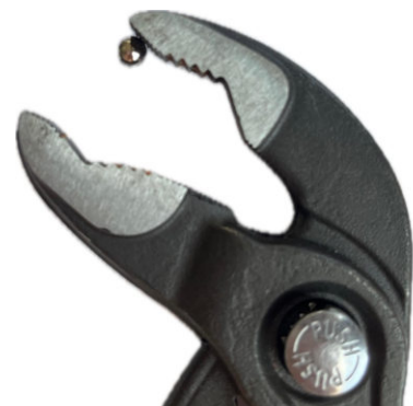
Fig. 7: Due to the ferromagnetic properties of the pipe wrench, the magnetic sphere adheres to it in the desired orientation
