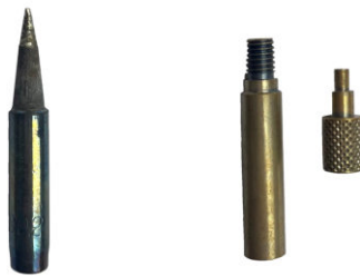
Fig. 11: Soldering tip (left) and tip for melting the thread inserts (right)
