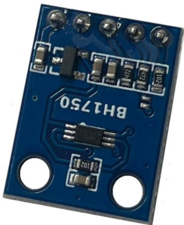
Fig. 6: Pin header soldered to the sensor
