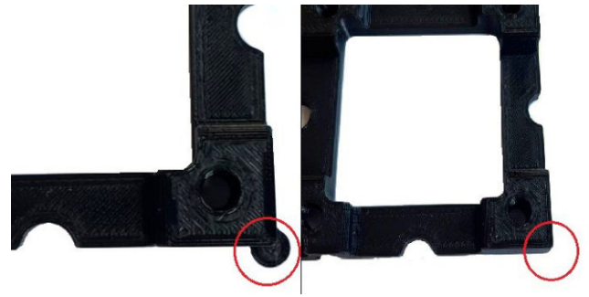
Fig. 5: Corner of the baseplate left before, right after removing the print residue, the red circles marks the corresponding areas
