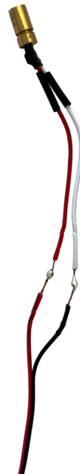
Fig. 12: Soldered cable with the laser diode
