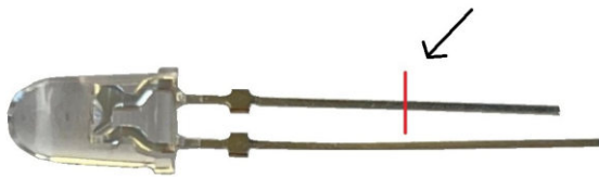
Fig. 9: Unshortened LED, the red marking shows the corresponding point at which the LED is to be shortened.
