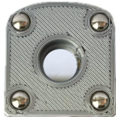
Fig. 7: Magnetic spheres pressed into the plate
