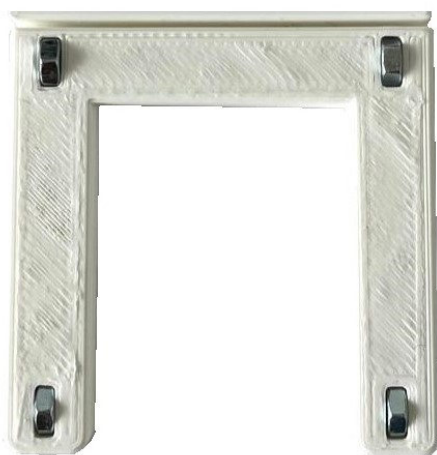
Fig. 8: Nuts in the base
