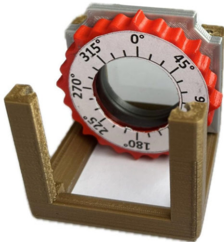
Fig. 11: Retaining and intermediate plate with the rotary wheel in the cube cover
