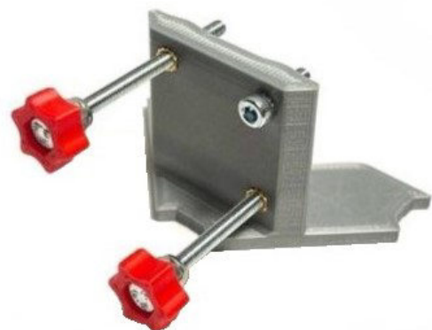
Fig. 6: Finished adjusting plate
