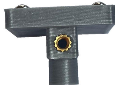
Fig. 8: Threaded insert melted into the LED plate
