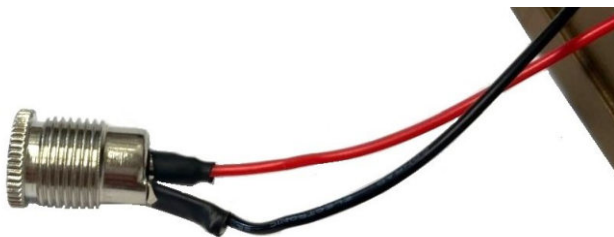
Fig. 20: Correctly connected DC-Socket
