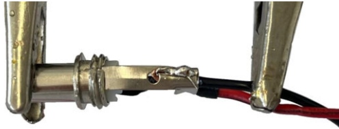
Fig. 16: Soldering the connector to the cable
