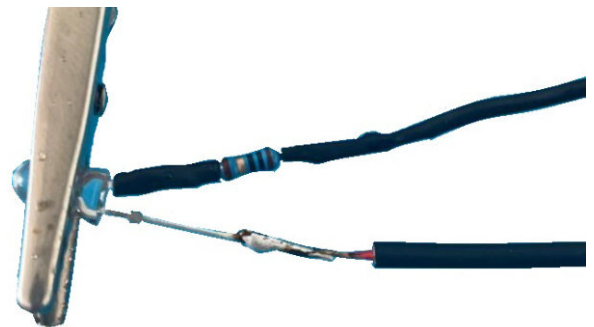
Fig. 14: Cables soldered to the LED
