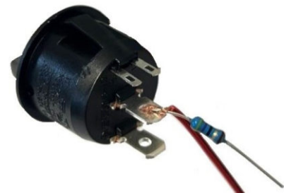
Fig. 5: Cable and resistor soldered to the changeover switch
