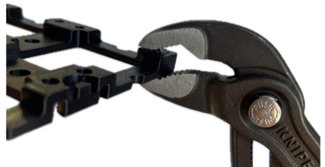
Fig. 6: Pressing in the magnetic spheres using a pipe wrench
