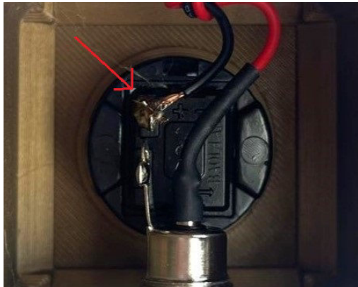
Fig. 7: Cable soldered to the button
