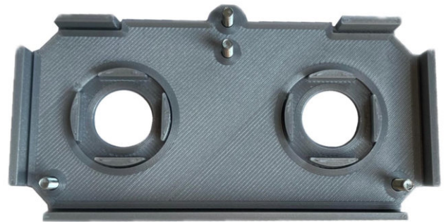
Fig. 10: Allen cylinder head screws pushed through the openings in the retaining and intermediate plate
