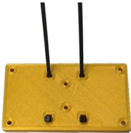
Fig. 23: Cable ties in the openings provided in the base
