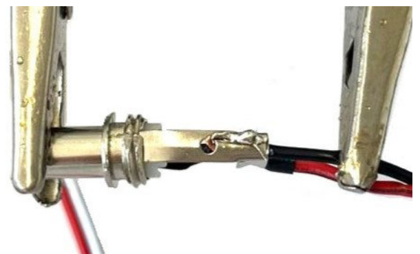
Fig. 10: Soldering the connector to the cable
