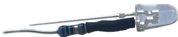
Fig. 12: LED soldered together with resistor
