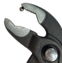
Fig. 16: Magnetic sphere sticks to ferromagnetic pliers
