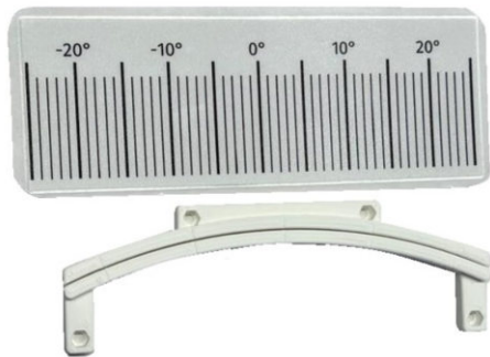
Fig. 4: Material required for the angular scale screen
