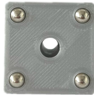
Fig. 7: Magnetic spheres pressed into the plate
