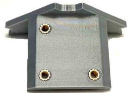
Fig. 5: Melting down the thread inserts
