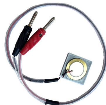
Fig. 16: Completely soldered piezo element
