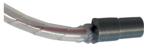
Fig. 19: Laser diode glued into the strain relief
