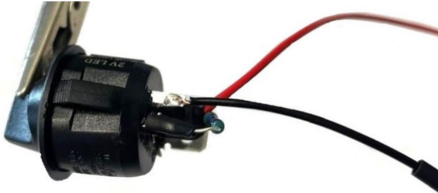
Fig. 8: Correctly soldered black cable
