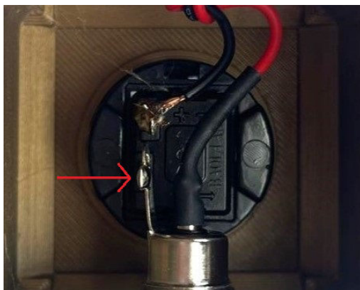
Fig. 8: DC-Socket soldered to the button
