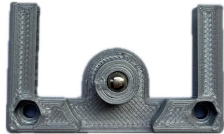
Fig. 4: Magnetic sphere pressed into the grating holder frame
