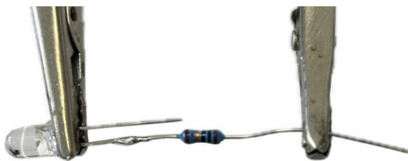
Fig. 11: Resistor soldered to the LED
