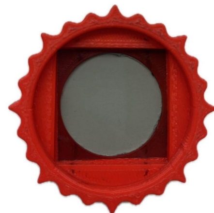
Fig. 5: Polarizing filter film inserted in the rotary wheel
