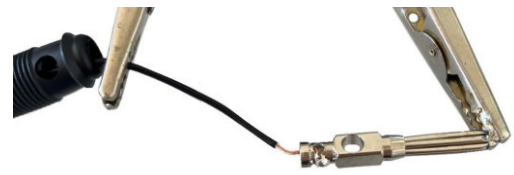
Fig. 12: Soldering the black cable to the banana black plug
