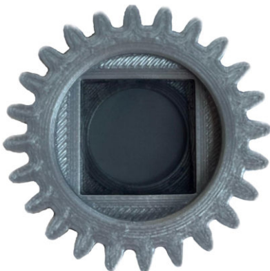
Fig. 4: Polarizing filter foil inserted in the wheel
