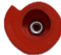
Fig. 11: Nut glued into the rotary button
