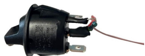
Fig. 7: Soldered resistor with heat-shrink tubing
