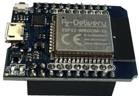
Fig. 4: Pin headers soldered to the PCB
