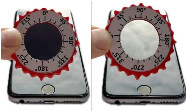
Fig. 6: Polarization on a glass plate (Brewster angle). The reflected light is absorbed on the left and transmitted on the right.
