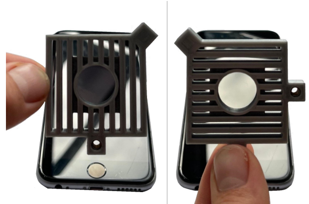
Fig. 10: Polarisation on a glass plate (Brewster angle). The reflected light is absorbed on the left and transmitted on the right.
