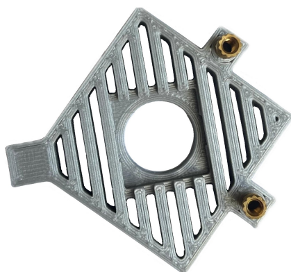
Fig. 4: Correctly positioned threaded inserts
