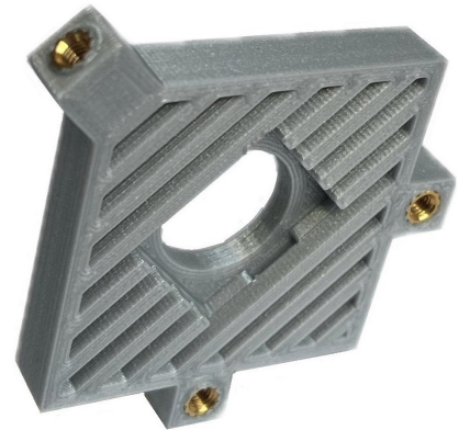
Fig. 6: Melted threaded inserts
